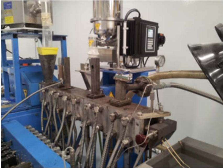
Figure 2. Coperion twin screw extruder the compounding process in AIMPLAS pilot plant.
